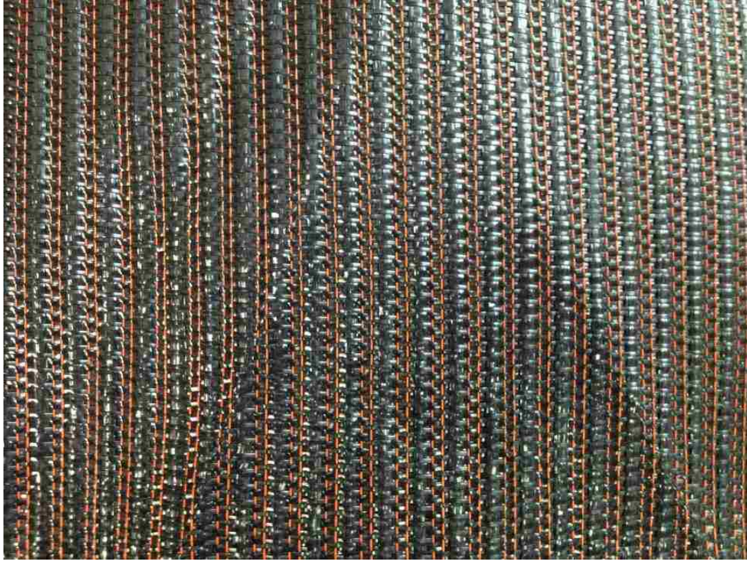
Figure 3-32. Photograph of the polypropylene Mirafi® RS380i fabric which was donated by Tencate Geosynthetics Americas for use in this GRS research study.
