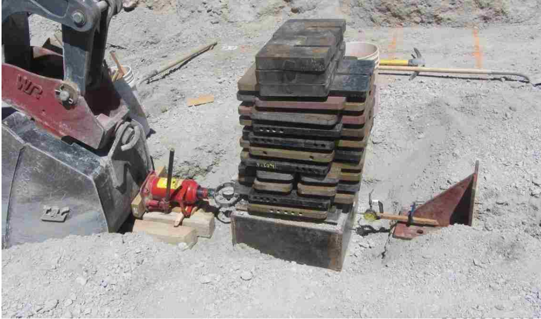
Figure 3-27. Photo of in-situ direct shear test on gravel backfill
